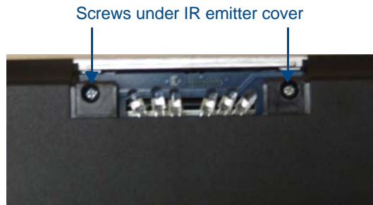
FIG. 114 Placement of screws underneath IR emitter cover
