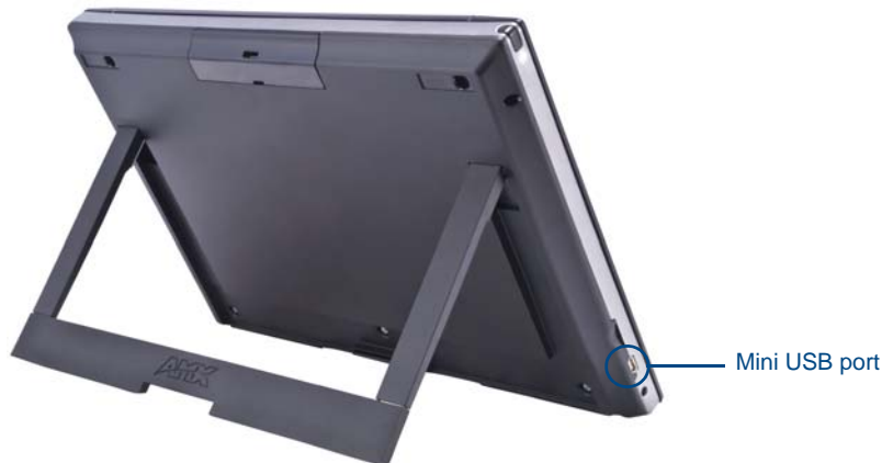
FIG. 29 USB Port on the MVP-9000i
