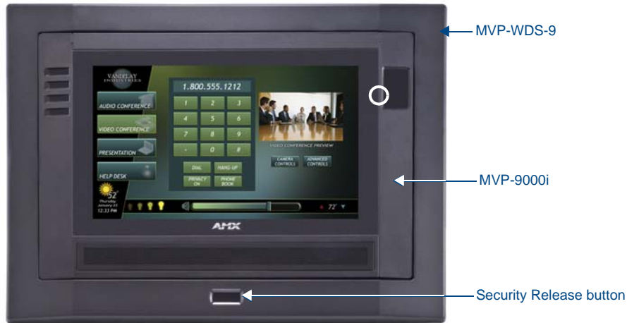
FIG. 10 MVP-WDS-9-GB Wall Docking Station - Front
